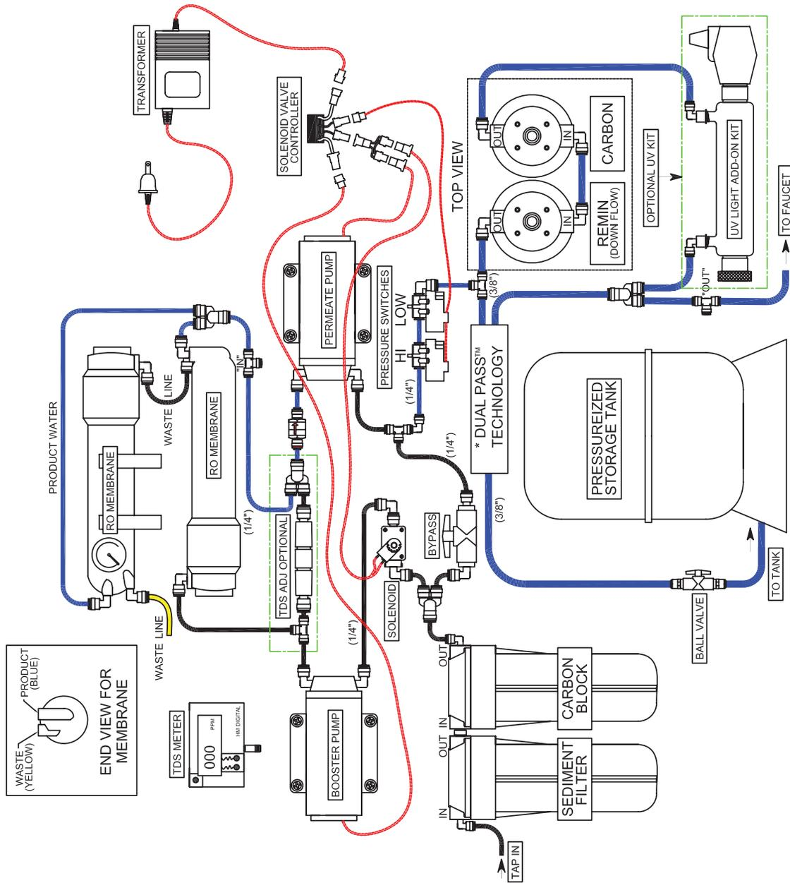
\* THIS SYSTEM HAS TWO 3/8" PRODUCT LINES. TO DETERMINE WHICH CONNECTS TO THE TANK AND WHICH TO THE FAUCET, FOLLOW THE BELOW PROCEDURE:
