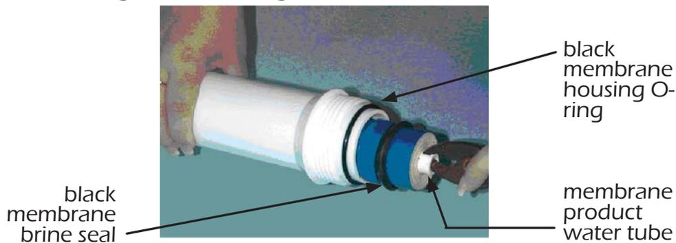
6. Remove the black housing O-ring (Fig. F). Wash the empty housing with soapy water. Rinse thoroughly with hot, clean water.
