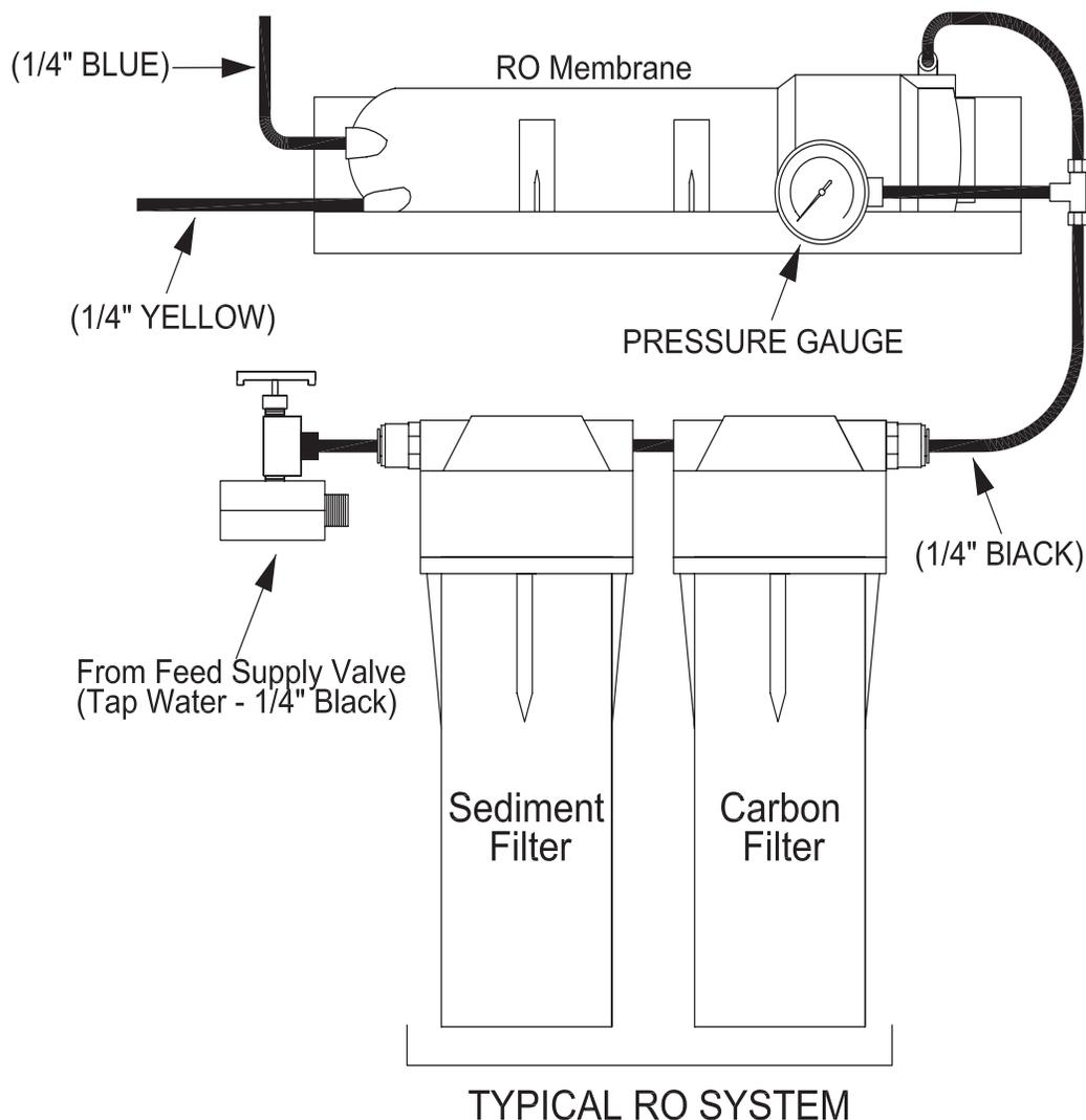
Figure 1: Installation of Pressure Gauge Kit .
