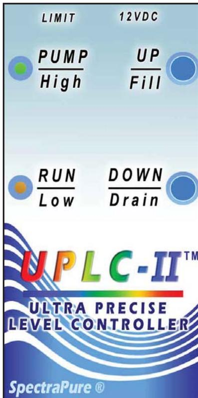
NOTE: In both cases, pressing the UP button directly after pressing the DOWN button will set the difference in levels to be minimal, typically less than 0.10"
